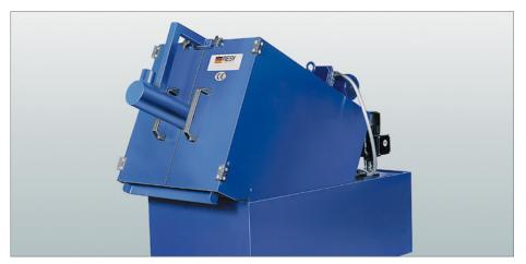
The RESY RSF roll screen filter system is used mainly as a standalone machine to remove chips from the filtering media. The filtration effect is varied by using different kind of filter fabrics.
